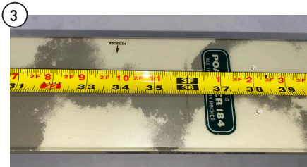
STEP 3: Verify the measurement on the tape measure corresponds with the midsole chart (Page 32-38).
